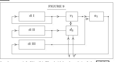
clearly have to contain d like elements (cf. {}). (b) The k (delay lengths) of the d l I d lIII. These too have certain functions of synchronization: Each time when the adder functions (that is in each interval it-ft) the multiplicand and the partial product sum (that is the outputs of d l I and of d lIII) must be brought together in such a manner that the former is advanced by t (moved by one position to the right) relatively to the latter, in comparison with their preceding encounter.
