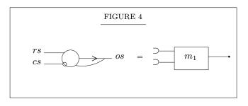
It should be noted that this <u>ml</u> corresponds to the actual vacuum tube trigger circuits mentioned at the beginning of 5.1. It is worth mentioning that <u>ml</u> contains one E-element, while the simplest trigger circuits contain one or two vacuum tubes (cf. loc. cit.), in agreement with the estimates of 6.5.
