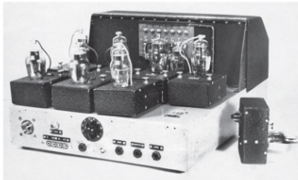
Delilah. Combining, power, and key units. The key unit is also shown with its top open to reveal the scrambler wheels at the rear and valves (one removed) at the front.
